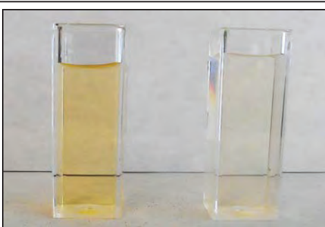
Figure 4. The sample on left is the dichromate solution without ethanol, and sample on right is the dichromate solution with ethanol.
