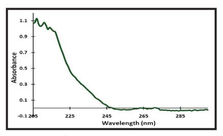
Figure 2: The UV/Vis Spectrum of THZ with a  $\lambda_{max}$  value at 208 nm
